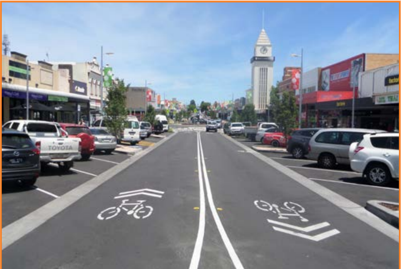
Figure 4.17 Shared-lane markings, traffic calming and lower posted speed limits have improved cycling safety through Warrnambool's town centre in regional Victoria.
