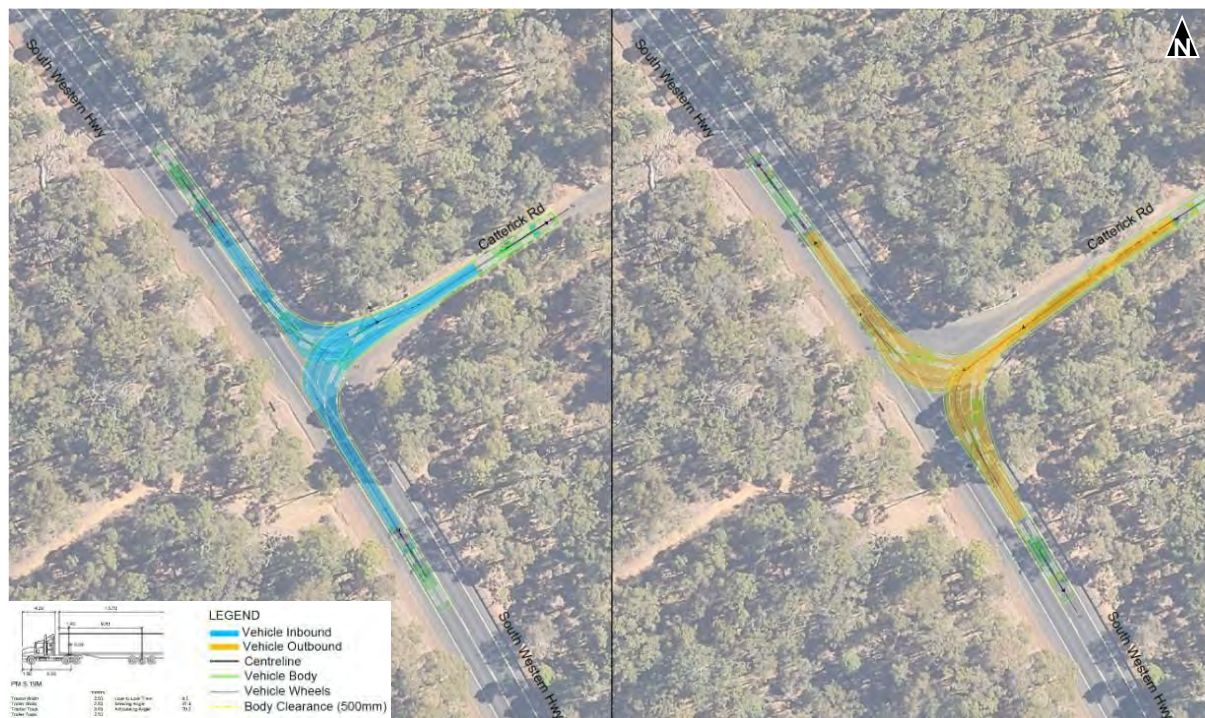
Figure 35 – Swept Path at Existing Intersection – 19.0m Truck
