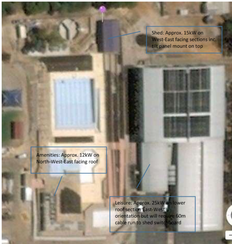
Figure 24 Available Roof space for solar PV supplying Pool
