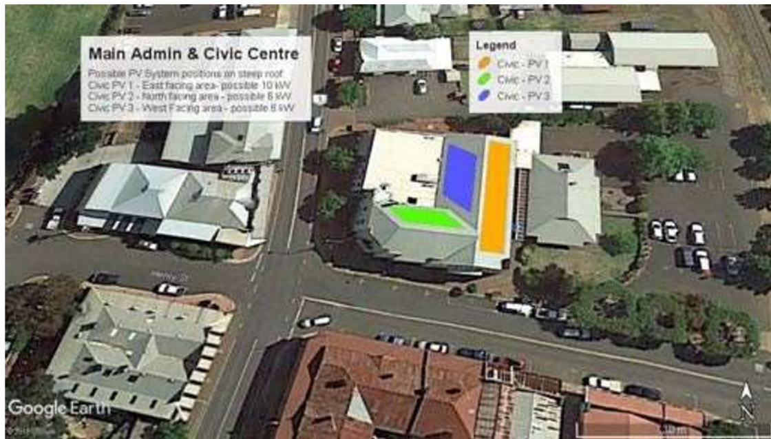
Figure 6 Admin Centre Solar PV Roof Space
