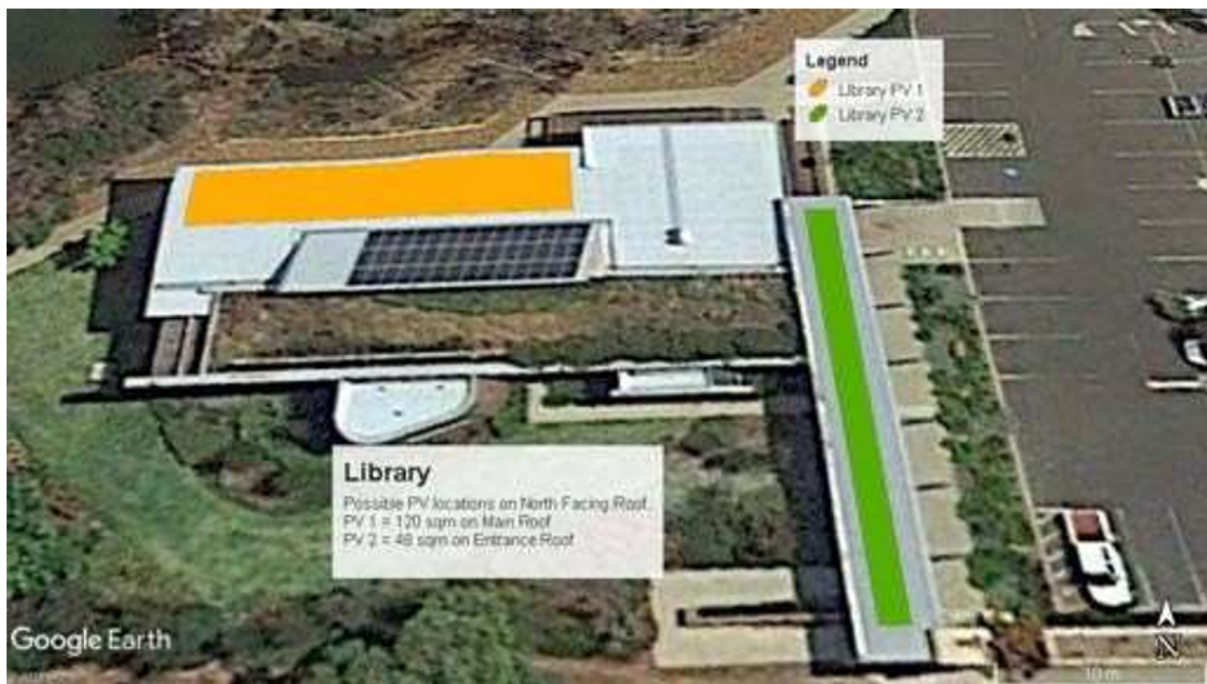
Figure 13 Library available roof space for solar PV
